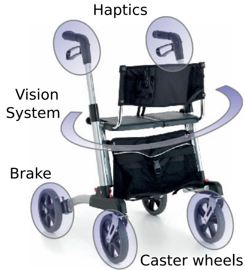
Fig. 1. Initial design of the mechanical guidance support (MGS).
